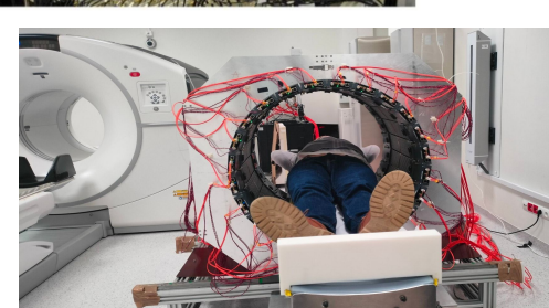
Figure 13. 24 modular J-PET, 2nd generation of J-PET tomography with 50 cm AFOV based on the SiPM (Completed 2021)
